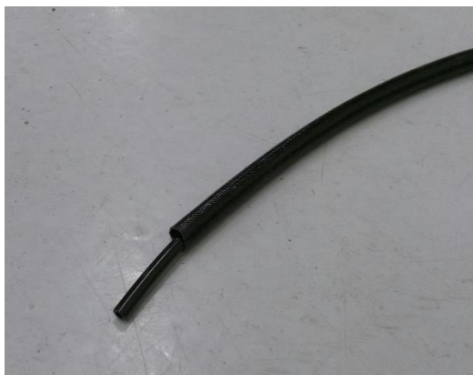
Figure 1 – Pipe in sleeve
